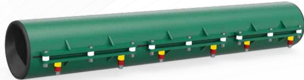
Roto's unique Wear Compensation Stator design allows to control and regulate the efficiency of Progressive Cavity Pumps for an extended period. It uses spacers (White, Yellow and Red colors) of engineered lengths to maintain even interference throughout the length of rotor and stator.
